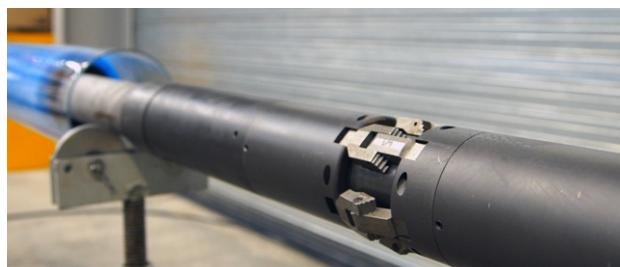
Filtrex, the One Trip Remedial Sand Control System, provides the flexibility to be installed thru tubing, through tight restrictions and expand into the casing ID filling all annular gaps regaining sand control. The first of its kind, the system provides the ability to perform sand clean out whilst installing the tool in one trip. Once set, the tool requires no further intervention.
