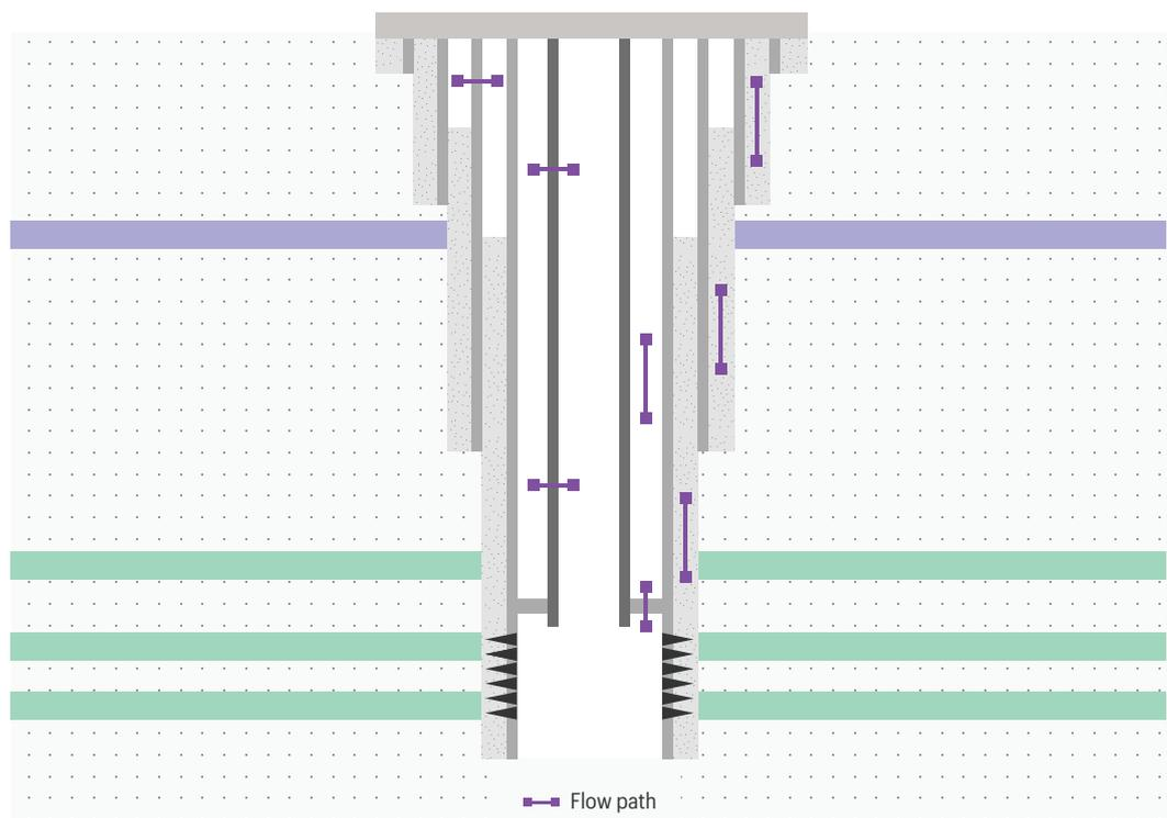
In the shut-in state, pressurised fluids from inside the tubing enter the A-annulus at three distinct points – X2000 ft, X4800 ft and X6400 ft. The fluid then enters the B- and C-annuli at X3600 ft via failures in the 7" and 9-5/8" casings. Fluid in the C-annulus then re-enters the formation via a failure in the 13-3/8" casing at X0900 ft.
